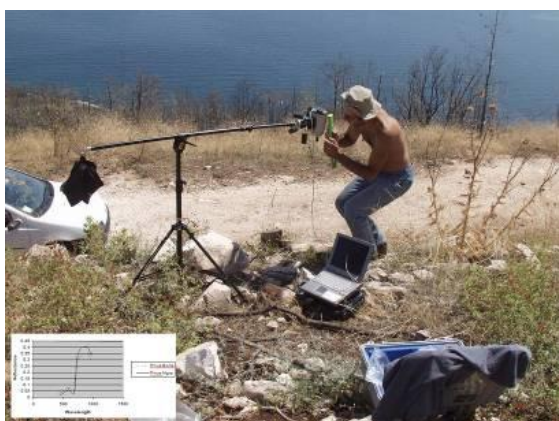
Field data collection with the use of spectroradiometer
